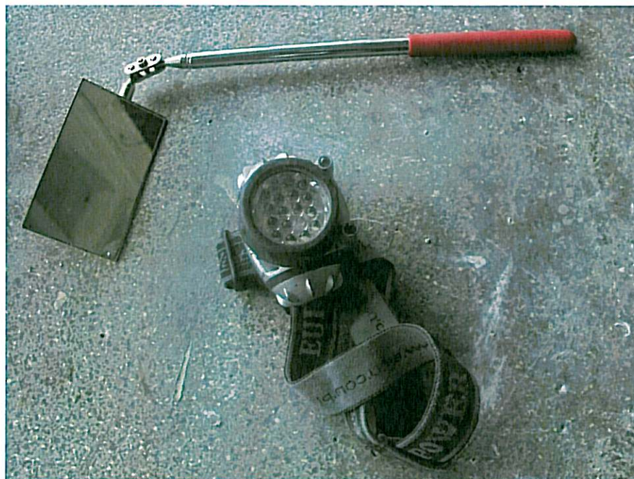
Figure 1. Inspection mirror and torch.
