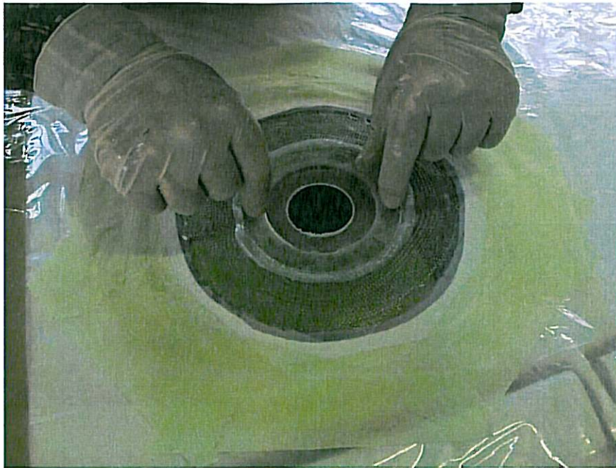
Figure 17. Press down the insert pad gently.
