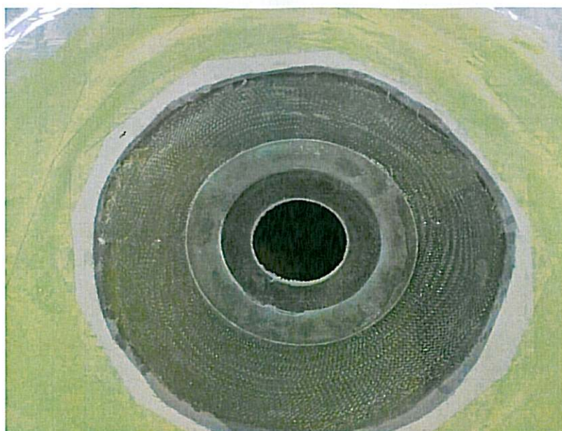
Figure 34. Insert pad before applying force.
