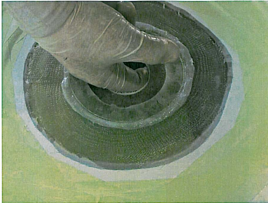
Figure 32. Removal of excess from wing inner surface.
