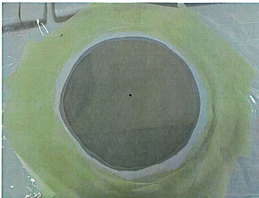
Figure 6. Removing paint and coating layers.
