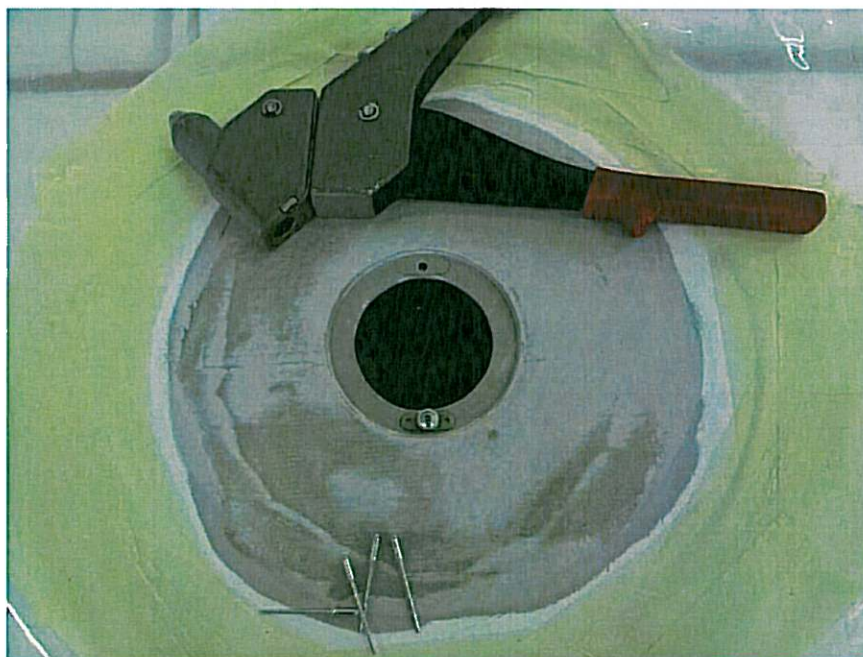
Figure 39. Kit for nuts mounting: anchor nuts - point 2, item. 8 + rivets - point 2, item 10 + Riveter - point 2, item 12.
