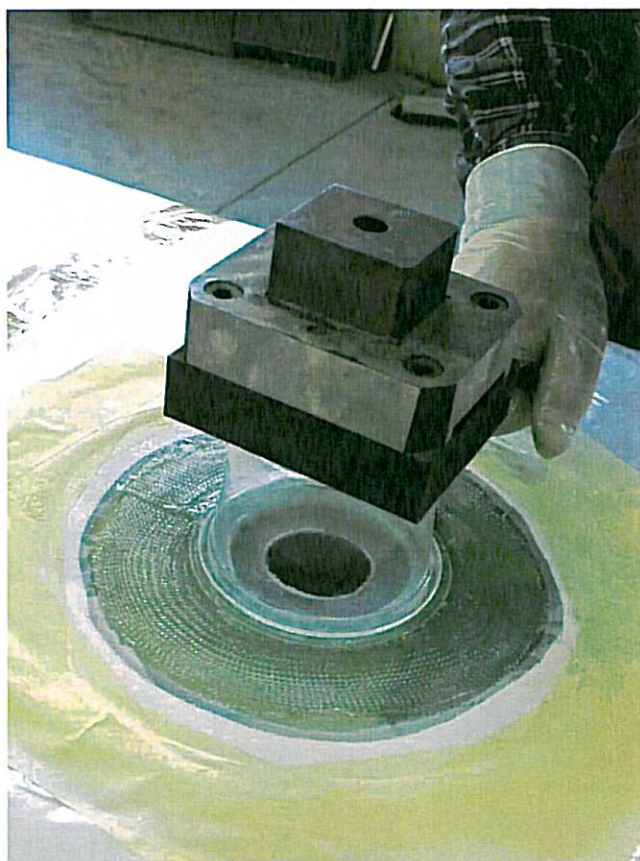
Figure 35. Insert pad loaded (max load 3 kg for 8 hours).
