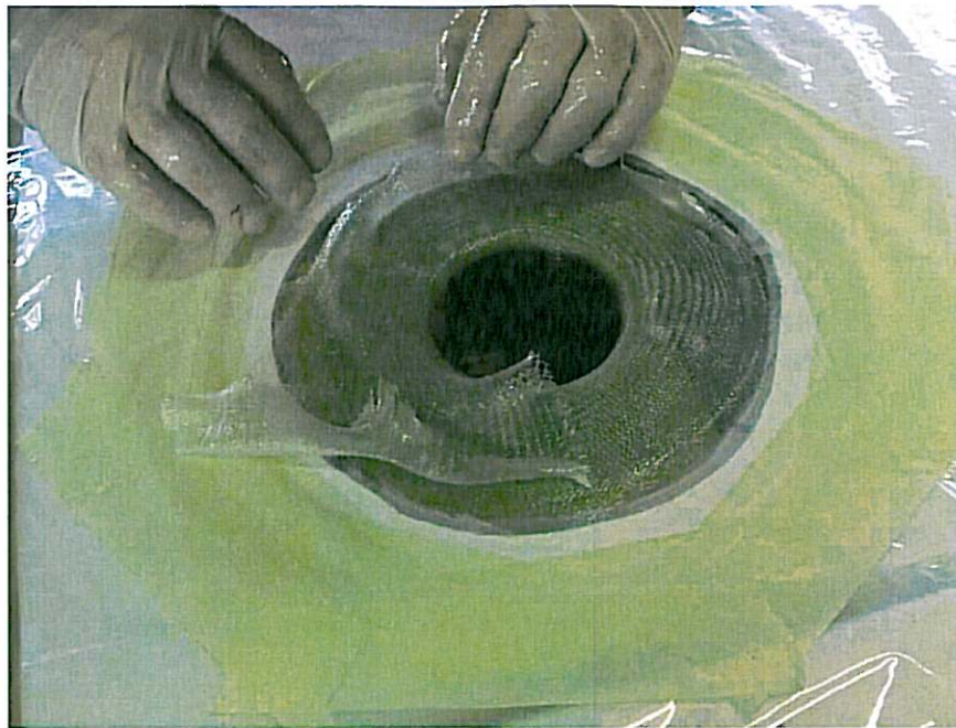
Figure 24. Placing layer 4... part 3.
