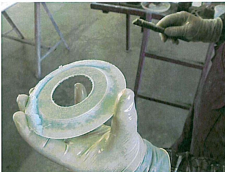
Figure 28. Application of gluing composition to insert pad
