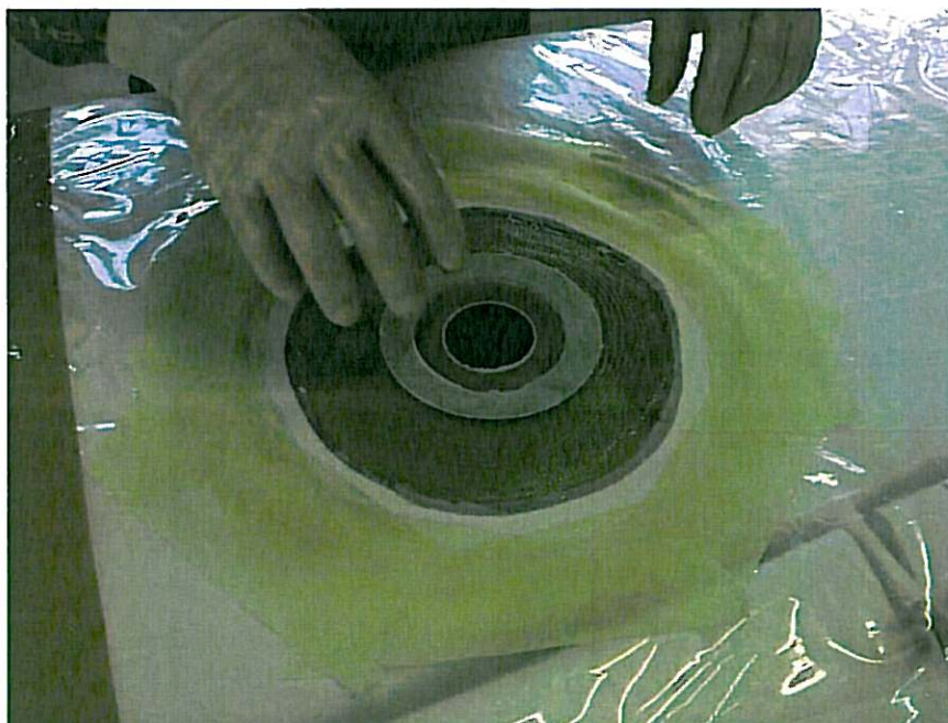
Figure 29. Embedding insert in the wing.
