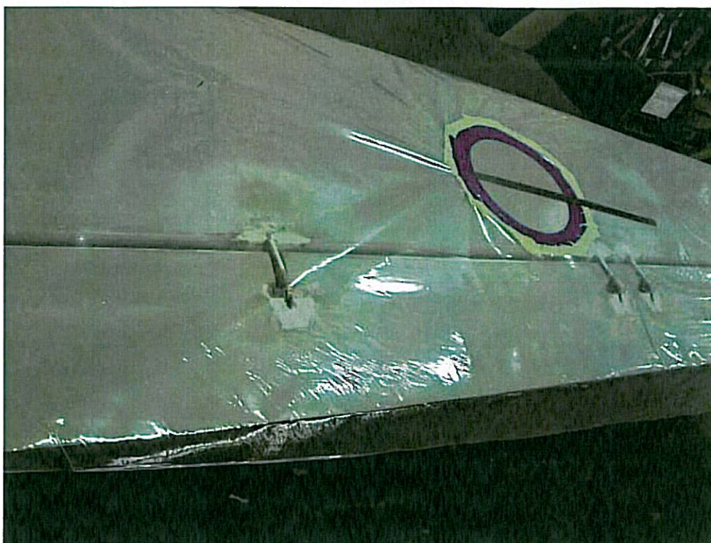
Figure. 4 Wing protection with foil
