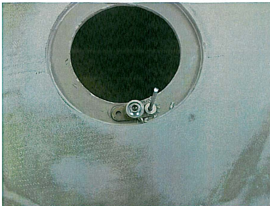
Figure 40. \varnothing 3 Hole drilling for nuts riveting, and chamfering for rivet head 1 \times 45^\circ - stage 1.
